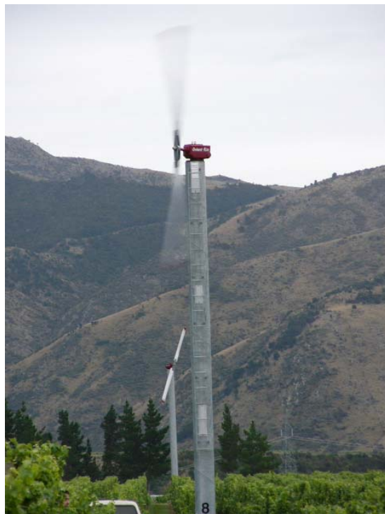
Orchard-rite wind machines similar to the 9 going in at Higgins Rd
